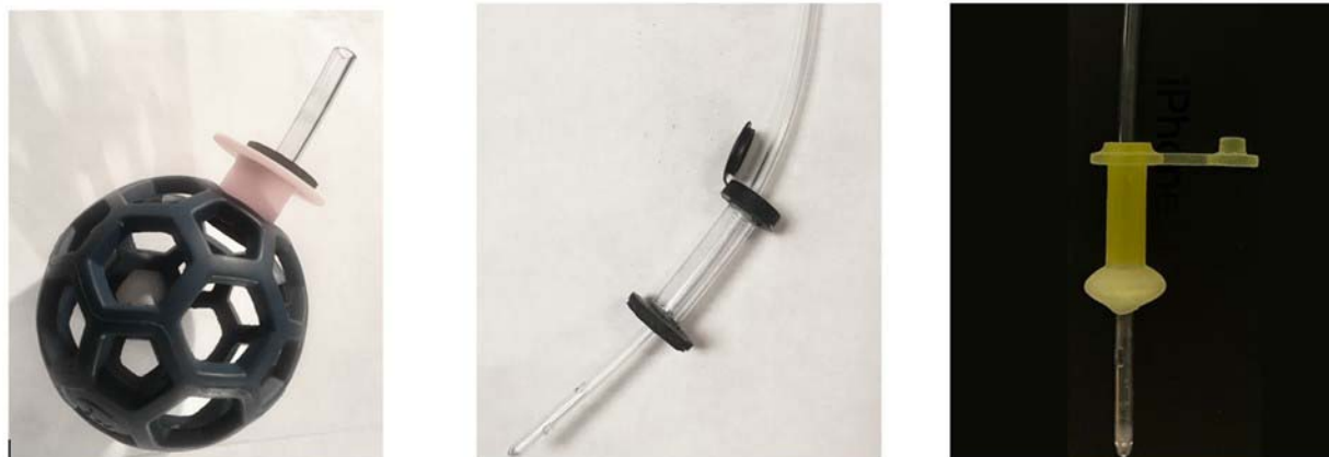
Figure 1: Early prototyping. Proof of concept can start anywhere. The earliest prototypes for the CathPort started with a dog toy and a trip to the hardware store.
